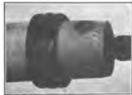
Fig. 172. Polishing Ring on Arbor.
